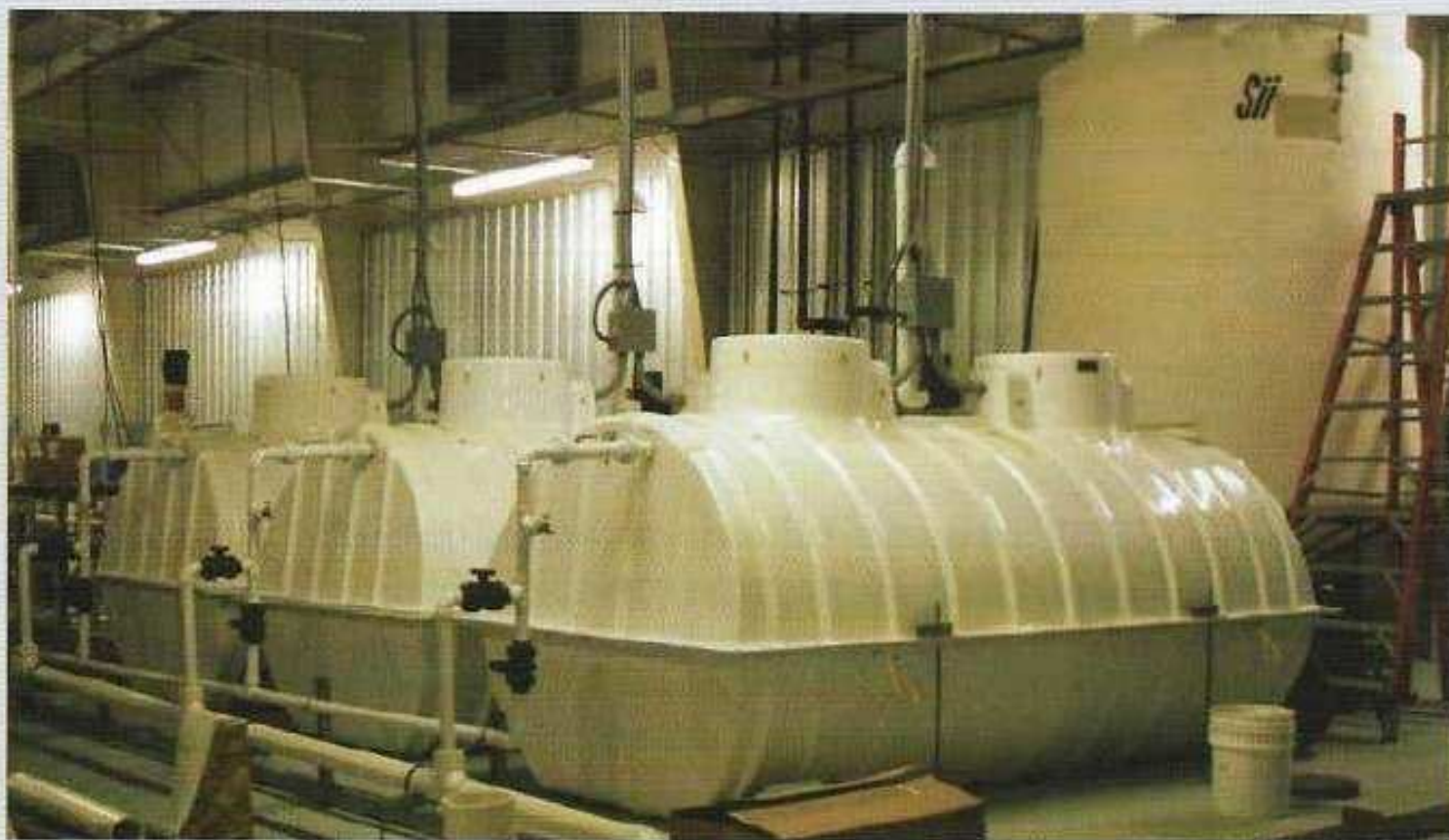
Figure 8.4: Three independent sequencing batch reactors used for experimental trials
