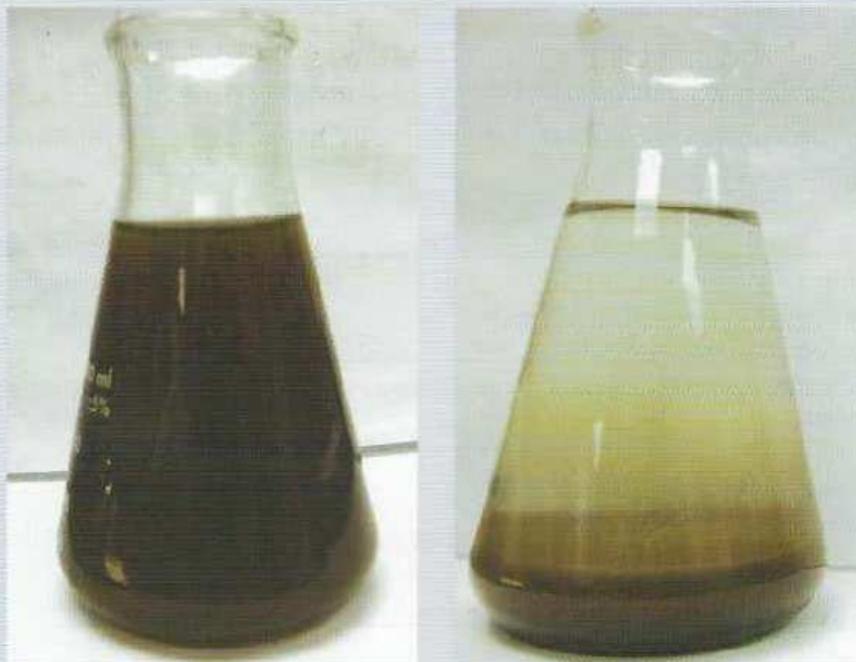
Figure 8.2: Untreated fish wastewater (left) compared to settled bioflocs after suspended-growth biological treatment (right)
