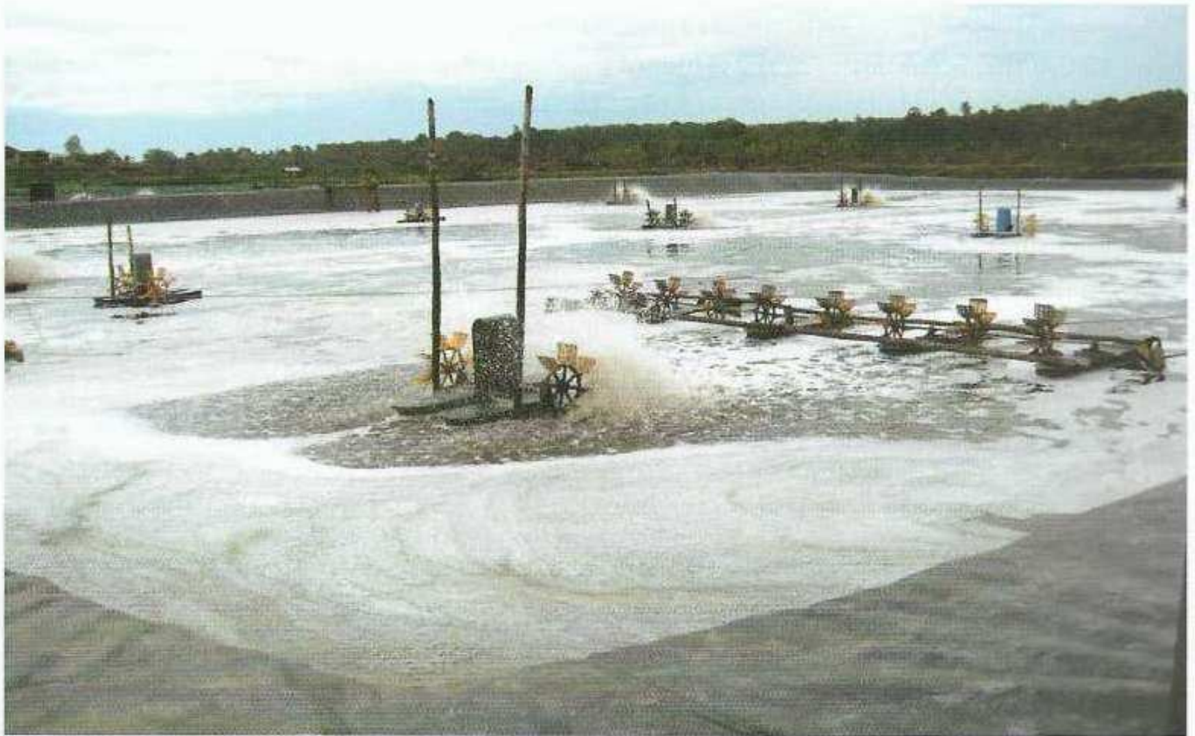
Figure 13.2: Aerated pond (Paddle wheels and long arm paddle wheel)
