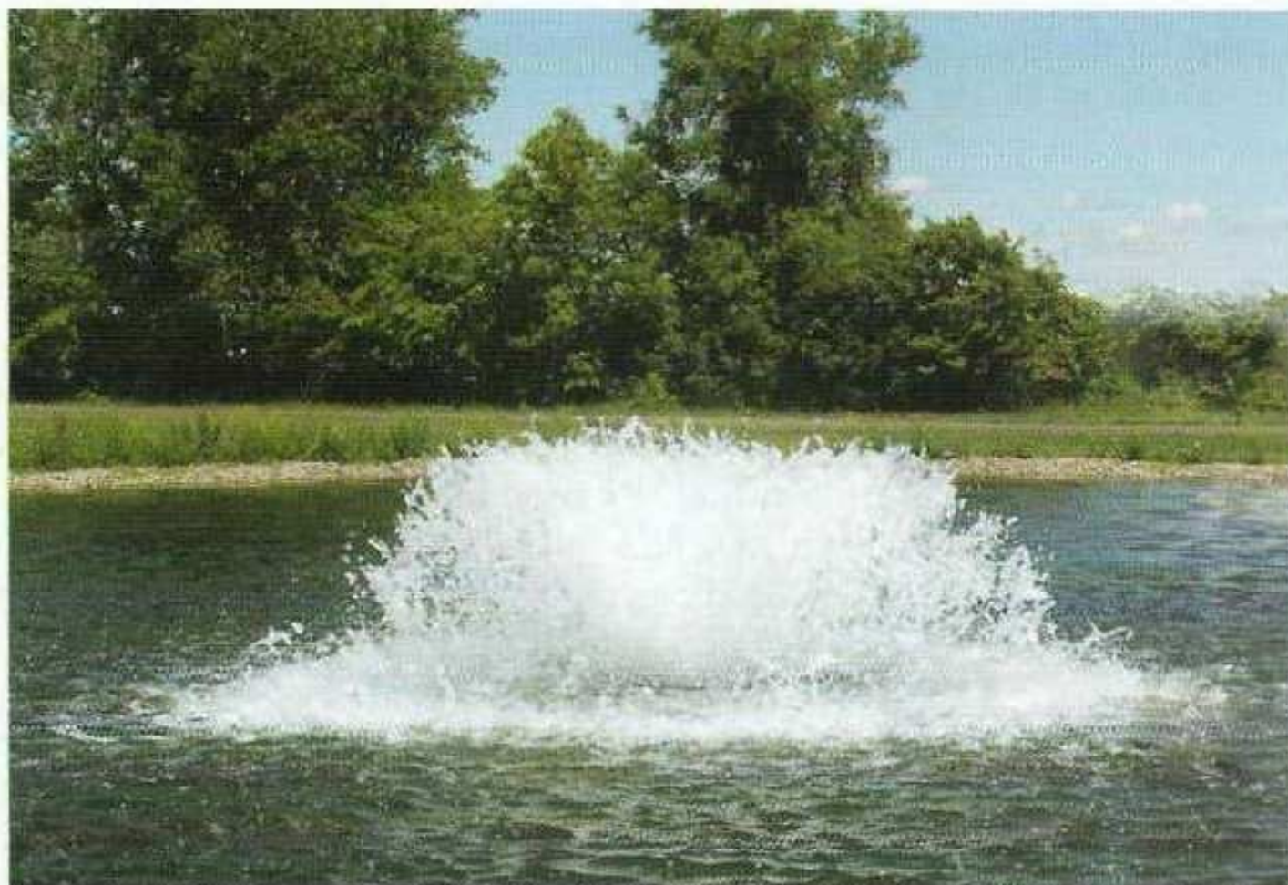
Figure 10.6 Vertical pump - Water is pumped upward with a submersible propeller and splashed onto the air.
